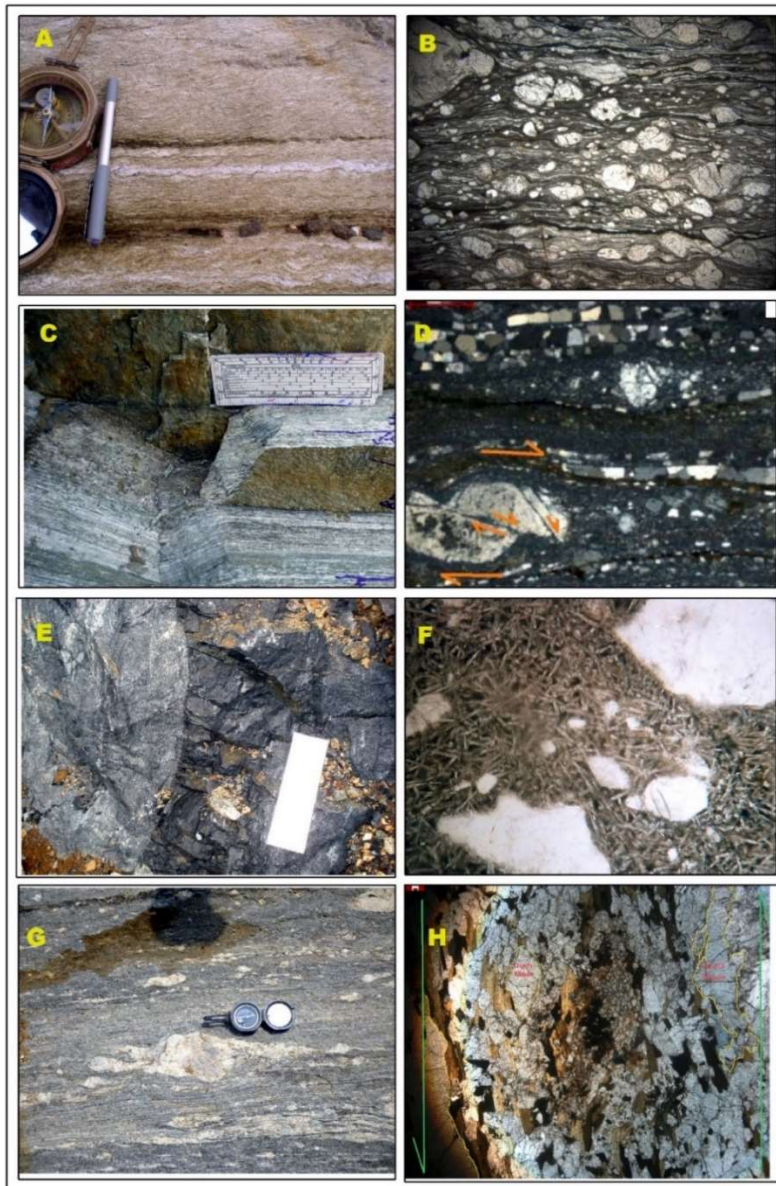
Figure 2 A. S-C Mylonite from Salem-Attur Shear Zone (SASZ), B. Porphyroclasts in thin section from Sarkar Natarmangalam, SASZ, C. Mylonites of Mettur Shear Zone (MSZ), D. Thin section of mylonite from MSZ- Fractured Porphyroclast displaying dextral sense. E. Pseudotachylyte in Charnockite from Gangavalli, GSZ, F. Microlites of albite in thin section of pseudotachylyte, Udayaturgate, GSZ, G. Sigmoidal porphyroclasts in mylonites from Tiruchengode, SKSZ, H. quartz ribbon in mylonites from SKSZ.
